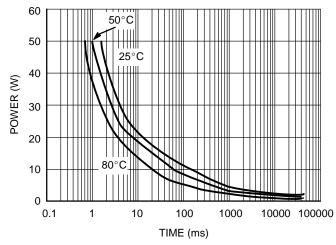
Figure 2. Power Dissipation vs. Thermal Trip Time
