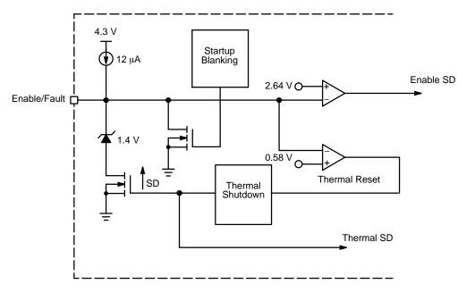
Figure 20. Enable/Fault Simplified Circuit
