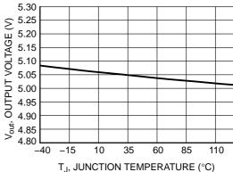
Figure 2. Output Voltage Variation with **Temperature**
