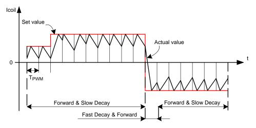
Figure 8. Forward and Slow/Fast Decay PWM
