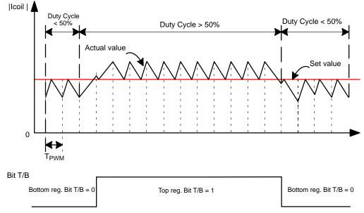
Figure 9. Automatic Duty Cycle Adaptation
