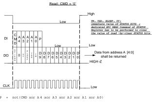
Figure 19. SPI Read Frame
