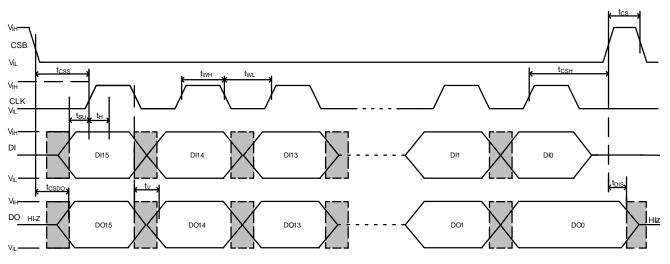
Figure 7. SPI Timing
