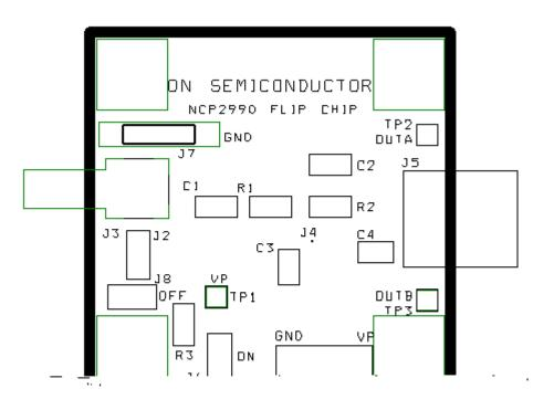
Figure 26. Demonstration Board for 9–Pin Flip–Chip CSP Device – Silkscreen Layers
