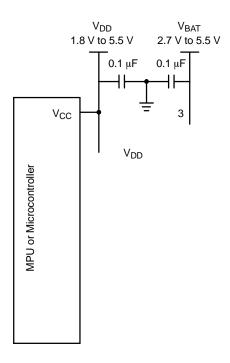
Figure 1. Typical Interface Application
