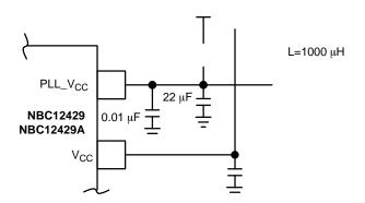
Figure 8. Power Supply Filter
