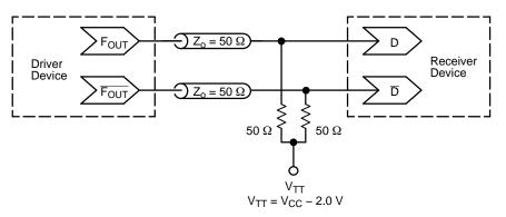
Figure 14. Typical Termination for Output Driver and Device Evaluation (See Application Note <u>AND8020/D</u> – Termination of ECL Logic Devices.)
