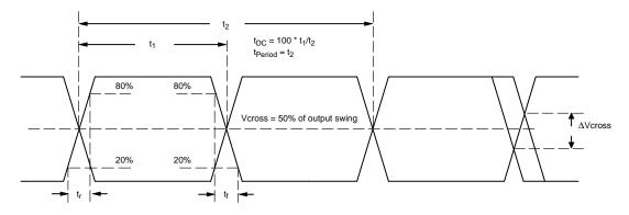
Figure 6. Differential Measurement for AC Parameters
