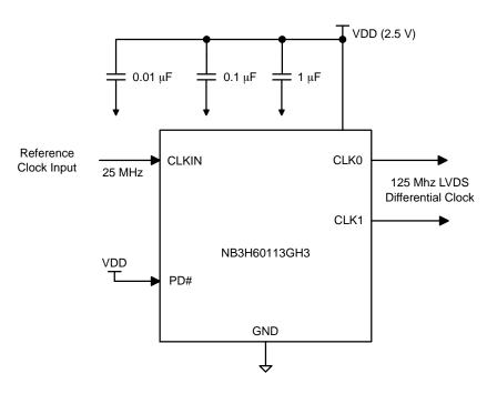
Figure 3. Power Supply Noise Suppression and Differential Output Application setup
