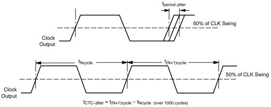
Figure 7. Period and Cycle-Cycle Jitter Measurement
