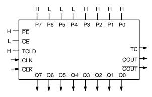
Figure 5. Mod 2 to 256 Programmable Divider
