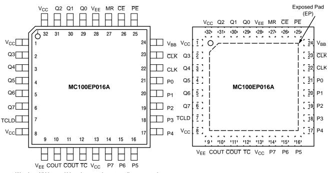
Warning: All  $V_{CC}$  and  $V_{EE}$  pins must be externally connected to Power Supply to guarantee proper operation.
