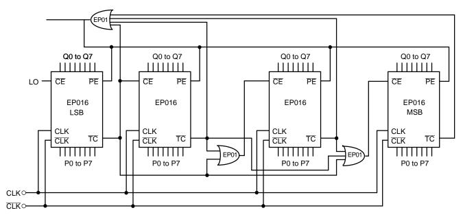
Figure 7. 32-Bit Cascaded EP016A Programmable Divider
