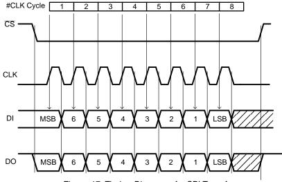
Figure 17. Timing Diagram of a SPI Transfer
